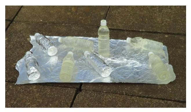
Figure 3.1 Experimental setup for testing disinfection process under sunlight.
